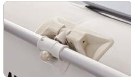
Built-in oar lock system for easy rowing
